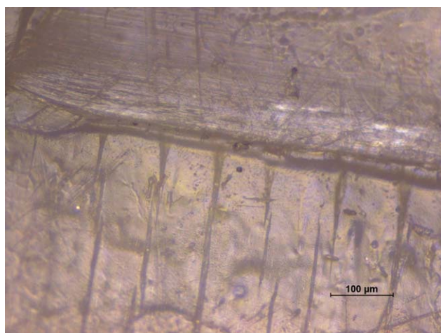
Figure 7. The optical micrograph (10× Nikon Eclipse 50i) of 9_140_300 after tensile test identifies the detached interface between tapes and vertical intratape cracks caused by load. [Color figure can be viewed in the online issue, which is available at wileyonlinelibrary.com .]
